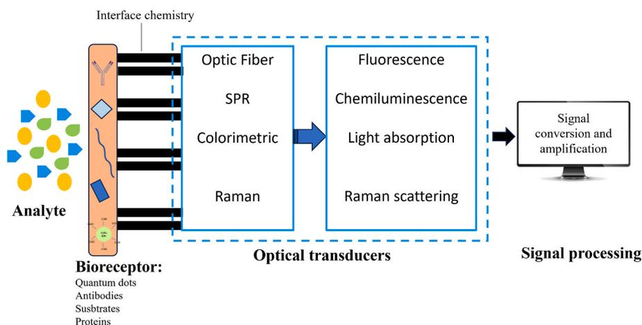
Fig. 6. Schematic representation of an optical sensor for the detection of biomarkers.
