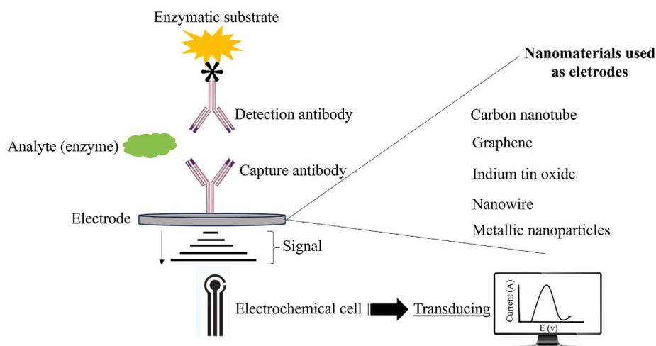
Fig. 8. Schematic representation of an electrochemical sensor developed for the detection of enzyme.
