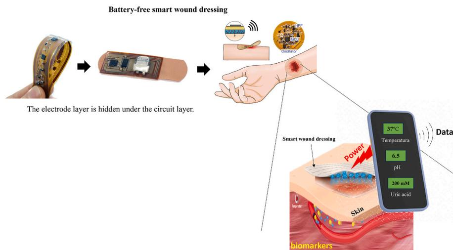
Fig. 4. Schematic representation of a battery-free sensor inserted into a wound dressing for the detection of biomarkers.
