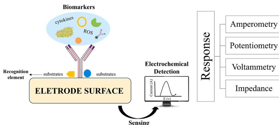
Fig. 5. Schematic representation of an electrochemical sensor for the detection of biomarkers.
