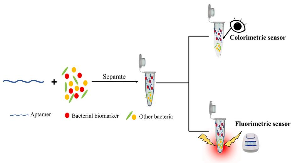
Fig. 7. Schematic representation of an optical sensor developed for the detection of bacteria.
